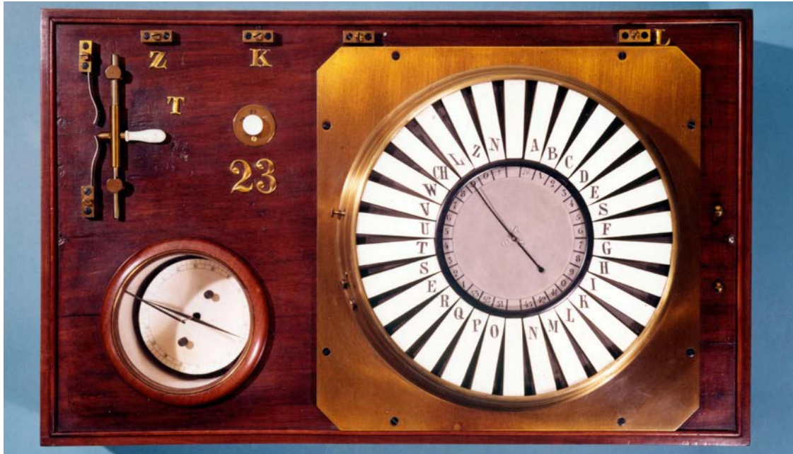
Dial telegraph invented by Werner von Siemens in 1847
